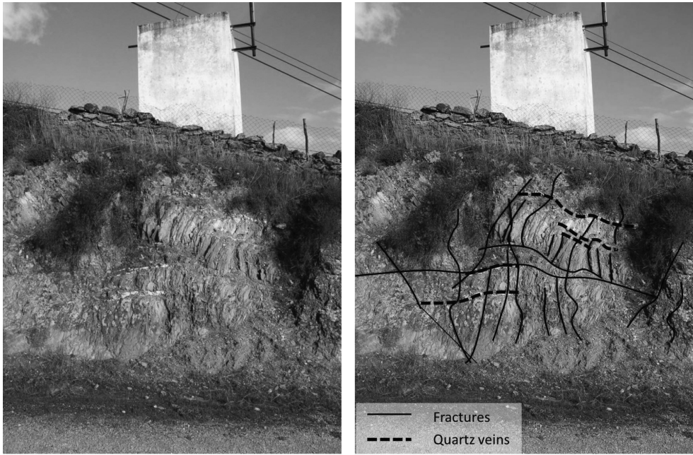
Figure 4.8 Example of a well in metamorphic rocks (shales, schists, greywackes) in central Portugal (area of Nisa). Quartz veins and fractures cut the rock in this specific position, where there is a productive well (yield of 8 l/s) which supplied a population of 70 inhabitants (the well is no more in use for water supply). (See colour plate section, Plate 13).
