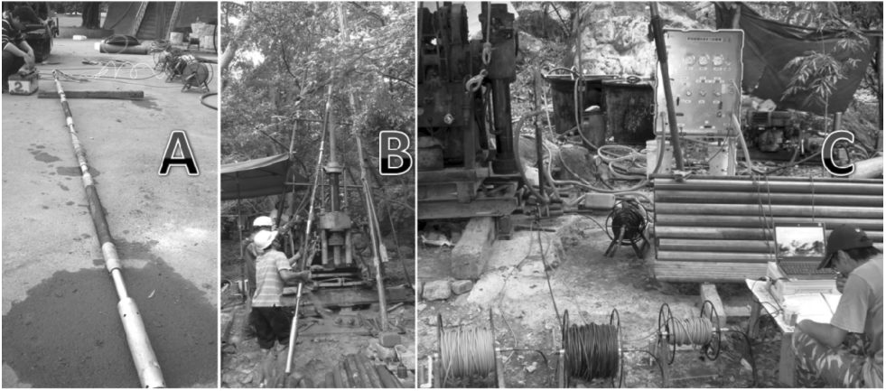
Figure 7.3 Photos taken during packer testing, (A) equipment calibration, (B) rig transfer, (C) data recording and analysis. (See colour plate section, Plate 23).
