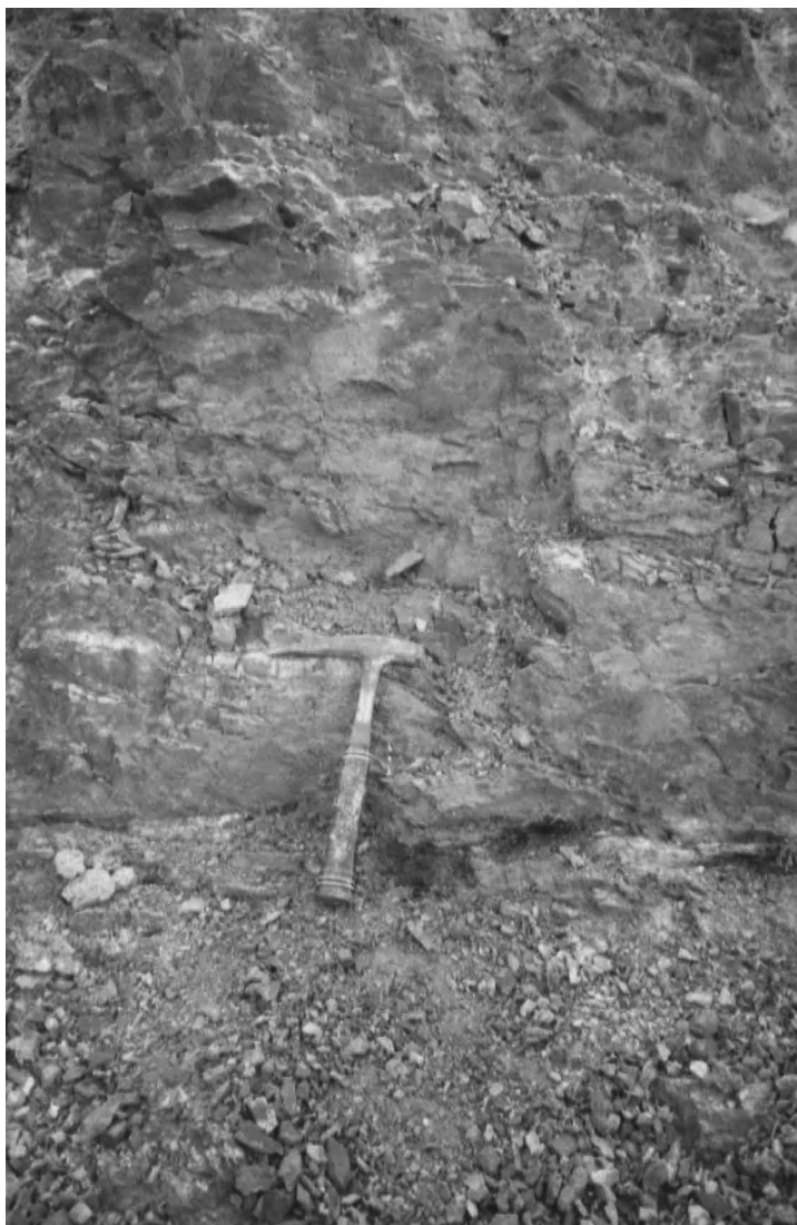
Figure 5.3 A granitoid outcrop showing the discontinuity network of the fissured layer. (See colour plate section, Plate 15).
