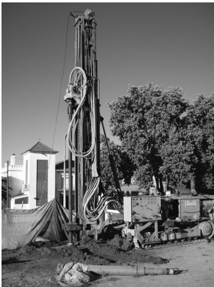
Figure 4.9 Drilling rig for rotary percussion. The compressed air enters the drill tubes (in the image near the top of the tower), and drives the percussion of the down-hole-hammer. The rotation of the hammer is given by the engine on the top of the drilling pipes.
