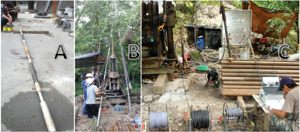
Plate 23 Photos taken during packer testing. (A) Equipment calibration, (B) Rig transfer, (C) Data recording and analysis. (see Fig. 7.3).
